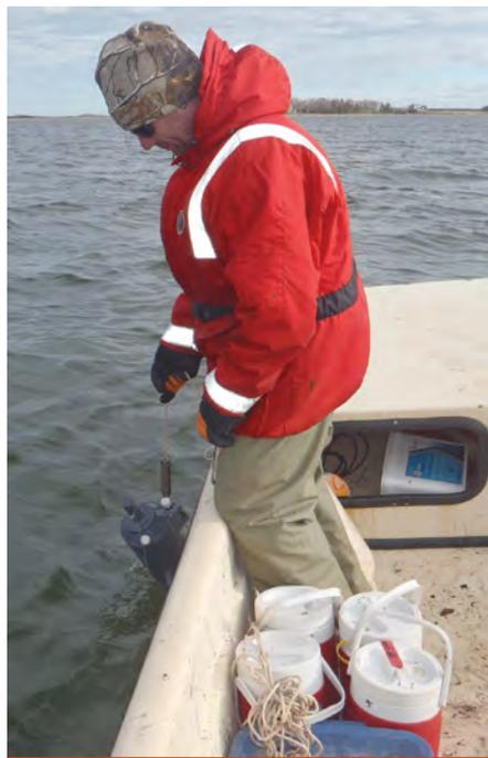
Collecting water samples for the measurement of primary production.
