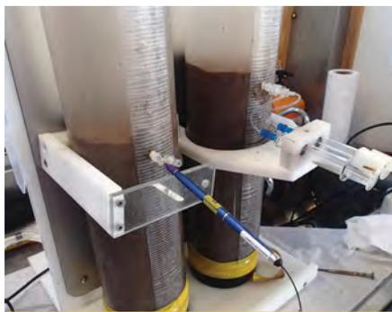
**Pore-water extraction and dissolved oxygen measurements being taken from sediment cores.**
