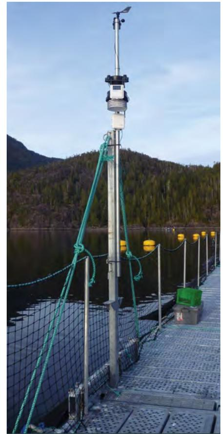
Davis weather station installed at fish farm in Clayoquot Sound providing real-time data via internet. Wind and solar radiation data are used as input to the FVCOM hydrodynamic model of the West coast of Vancouver Island.
