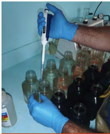
Measurement of primary production by injecting a stable isotope tracer.
