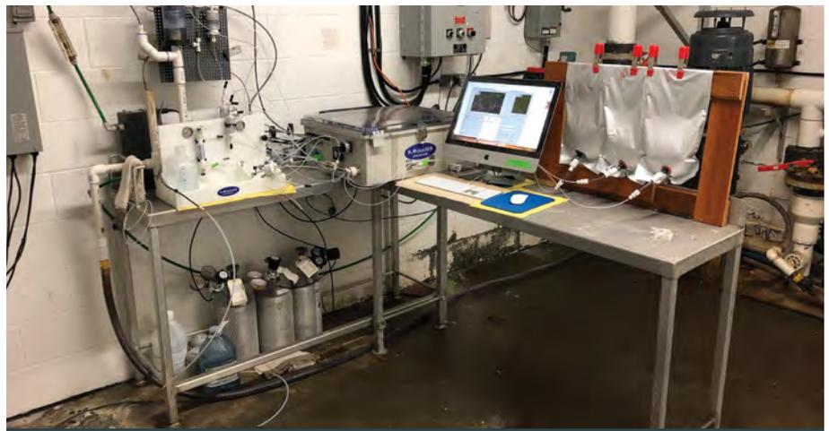
The BCSGA Burke-O-Lator (BoL) pCO<sub>2</sub>/TCO<sub>2</sub> analyzer, installed at Fanny Bay Oysters in Baynes Sound, tracks seawater CO<sub>2</sub> content.
