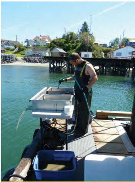
Macrofauna being extracted from benthic mud using running water and a sieve.
