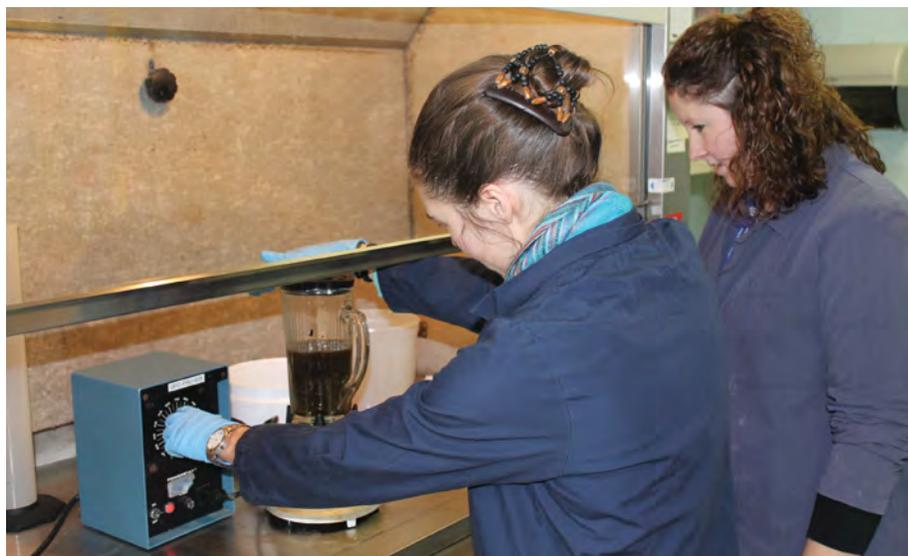
Homogenisation of benthic samples prior to DNA extraction and metabarcoding.
