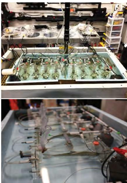
An overview (top) and a detailed view (bottom) of 8-channel automatic intermittent-flow respirometry system to measure integrated respiratory assessment paradigm (IRAP).
