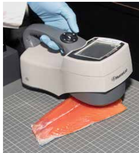
Colourimeter used to measure the colour in salmon fillets. Photo: Sébastien Plante (UMCS)
