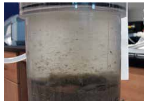
In-laboratory erosion measurements of mussel aquaculture waste using a Gust microcosm erosion chamber and a sandy seabed. Applied bed shear stress of 0.08 Pa is strong enough to mobilize the waste material and re-suspend large aggregates. Photo: Particle Dynamics Lab, BIO (DFO)
