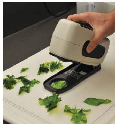
Fragments of the green alga, Ulva lactuca , analyzed for their colour with a handheld colour spectrometer as a means of monitoring dissolved nutrients. Photo: Andrew Cooper (DFO)
