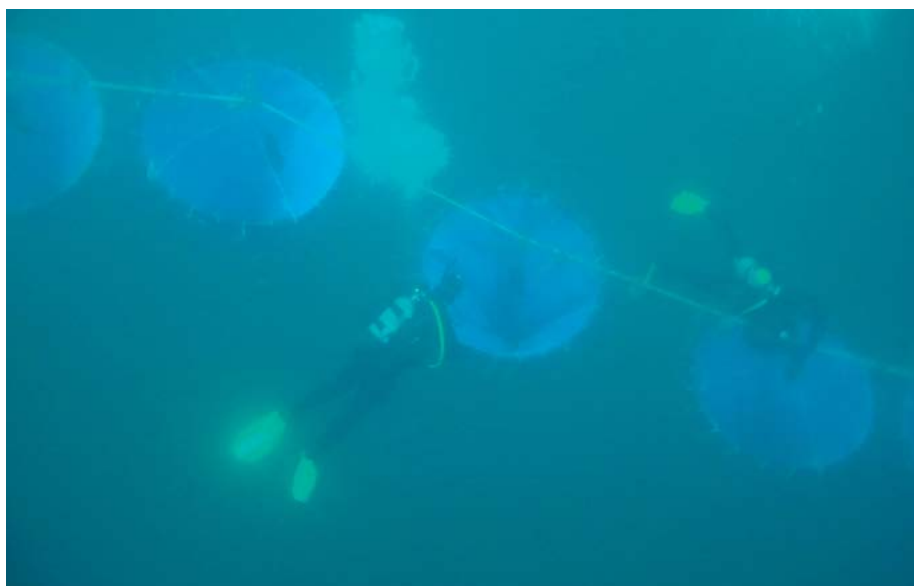
Divers work on large sediment traps to measure bio-deposit production by farmed mussels in Îles de la Madeleine. Photo: François Roy (DFO)
