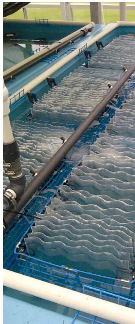
Fiberglass plates that will be used for the settling of larval sea urchins once they are produced in the hatchery and are ready for metamorphosis. Photo: Shawn Robinson (DFO)
