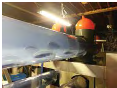
Exercise training Atlantic Salmon ( Salmo salar ) in the Brett-type two-channel swimming tunnel. Photo: Yangfan Zhang (UBC)
