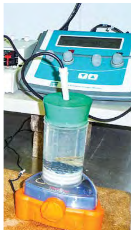
Respirometry system for measuring the physiological status of bivalves. Photo: Lisandre Gilmore-Solomon (Merinov; CÉGEP de la Gaspésie et des Îles)
