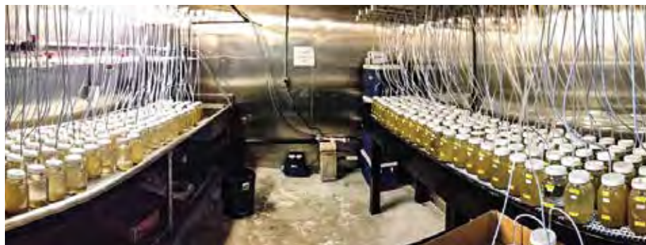
Stage V lobsters exposed to sediment spiked with ivermectin and emamectin benzoate using commercial formulations in thermoregulated room. Photo: HMSC
