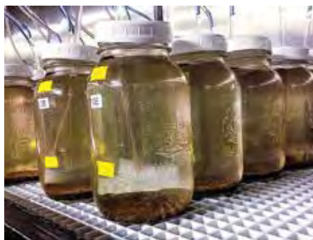
Aerated jar with stage V lobster exposed to sediment spiked with emamectin benzoate using commercial formulation. Photo: HMSC
