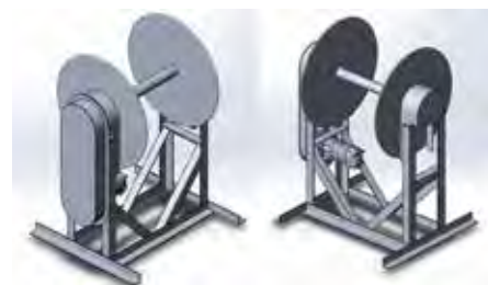
Design drawings of a rotating drum with a hydraulic motor. Photo: Daniel Leblanc (Merinov)
