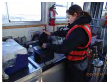
Lindsay Brager (DFO) conducting field tests of a new method for rapidly and accurately measuring sediment sulfide concentrations. Photo: Peter Cranford (DFO)
