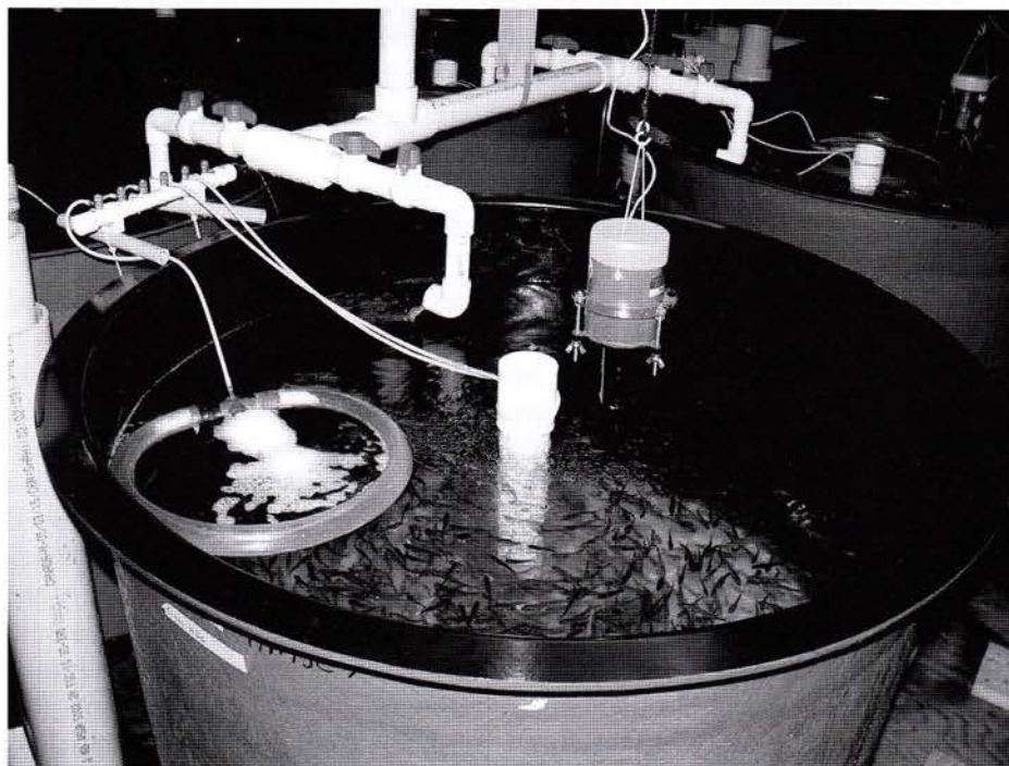
Figure 3 470 L individual family rearing tank (post-hatch to PIT-tagging) with automatic feeder.
