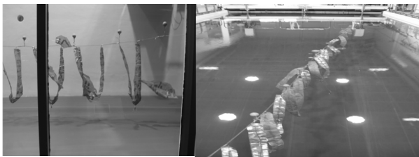
Figure 2. Longline set-up in MI flume tank. Floats are approximately 1 meter apart in the model.
