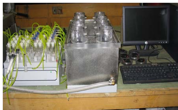
Figure 1. Laboratory setup showing respirometer system with compost columns.
