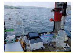
Part of the field set-up for measurement of total free sulfides, shown here during sampling at a shellfish site. Photo: Lindsay Brager (DFO)
