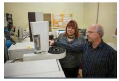
Dr. Chis Parrish and Jeanette Wells place a sample vial in a gas chromatograph's autosampler, which is used to determine fatty acids in lipid extracts. Photo: Genome Canada
