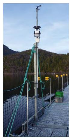
Davis weather station installed at fish farm in Clayoquot Sound providing real-time data via internet. Wind and solar radiation data are used as input to the FVCOM hydrodynamic model of the West coast of Vancouver Island. Photo: Glenn Cooper (DFO)
