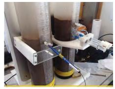
Pore-water extraction and dissolved oxygen measurements being taken from sediment cores. Photo: Peter Cranford (DFO)
