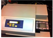
Blood samples contained in the tonometer (left). The tonometer is then placed in the spectrophotometer (right) to quantify the oxygen equilibrium curve of hemoglobin. Photo: Phillip R. Morrison (UBC)
