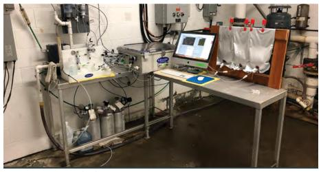
The BCSGA Burke-O-Lator (BoL)  $pCO_2/TCO_2$  analyzer, installed at Fanny Bay Oysters in Baynes Sound, tracks seawater  $CO_2$  content. Photo: Wiley Evans (Hakai Institute)
