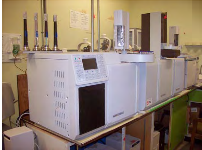
Varian 3800 GC-FID used to obtain FAA peaks.
